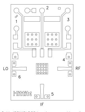
The grounded Co-Planar Wave Guide (CPWG) PCB input/output transitions allow use of Ground-Signal-Ground (GSG) probes for testing. Suggested probe pitch is 400 mm (16 mils). Alternatively, the board can be mounted in a metal housing with 2.4 mm coaxial connectors.
